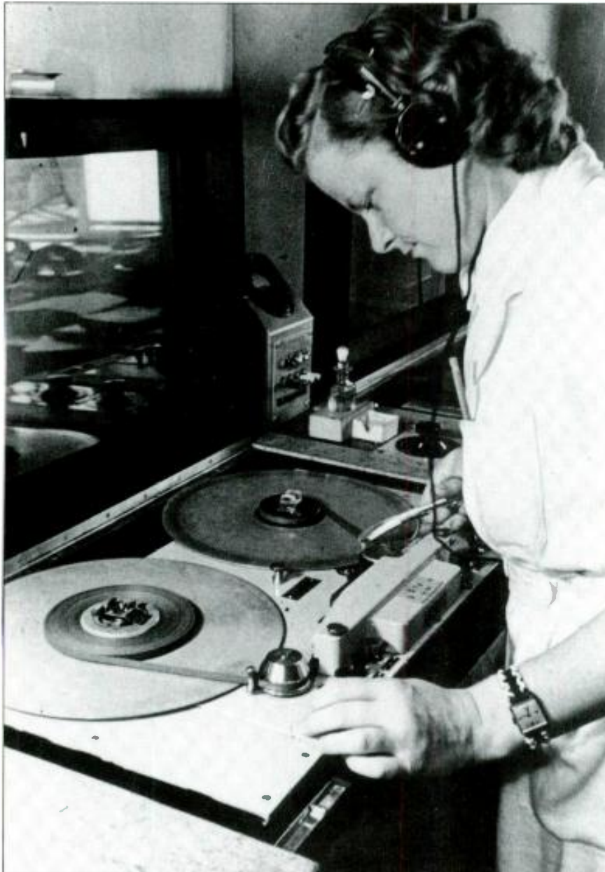
Figure 1. At a WWII Radio Stuttgart installation, an operator threads a Magnetophone tape recorder. Photo courtesy The Pavék Museum.
